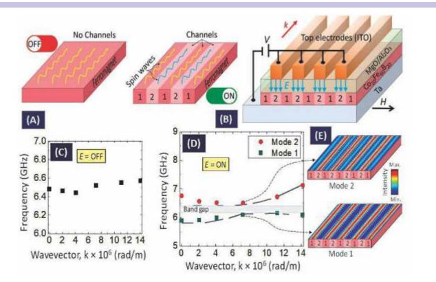
Fig. 1: A. Schematic illustration shows the concept of spin wave nanochannels. B. Schematic illustration shows the device structure and formation of nanochannels. Spin-wave frequencies versus wavevector when electric field, E is OFF (C) and ON (D). E. Heatmap plots show the spatial distribution of spin-wave intensity for spin-wave mode 2 and mode 1 at wavevector  $k = 7.1 \times 10^6$  rad/m.
