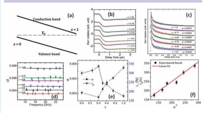
**Fig. 2:** A. Schematic of composition-dependent band structure of CEMS Heusler alloy. Time-resolved B. ultrafast demagnetization and C. precessional dynamics. D. Damping as a function of frequency. E. Variation of damping and demagnetization time with composition. F. Correlation between demagnetization time and damping.
